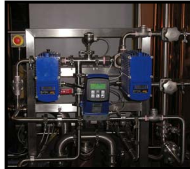
Emech F2-025 and F2-040 using 3 rd party actuation
